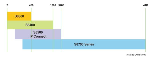
Figure 4: Avaya Application Solutions platforms port capacities
